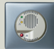
GAS AND FLOOD DETECTOR Identification of gas or water leaks, transmission of warning signal and closing-off of the incoming gas supply by solenoid valve
